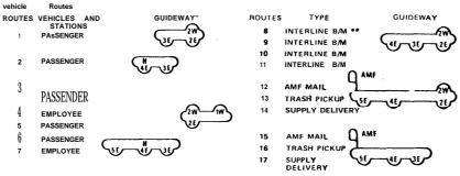
PASSENGER VEHICLES WILL USE THE PASSENGER (INSIDE) ROUTE OF THE GUIDEWAY THROUGH THE TERMINALS ALL OTHER VEHICLES WILL USE THE OPPOSITE (OUTSIDE) ROUTE OF THE GUIDEWAY THROUGH THE TERMINALS INTERLINE BM ROUTES DIFFER IN LOADUNLOAD FUNCTION AT EACH STATION.
