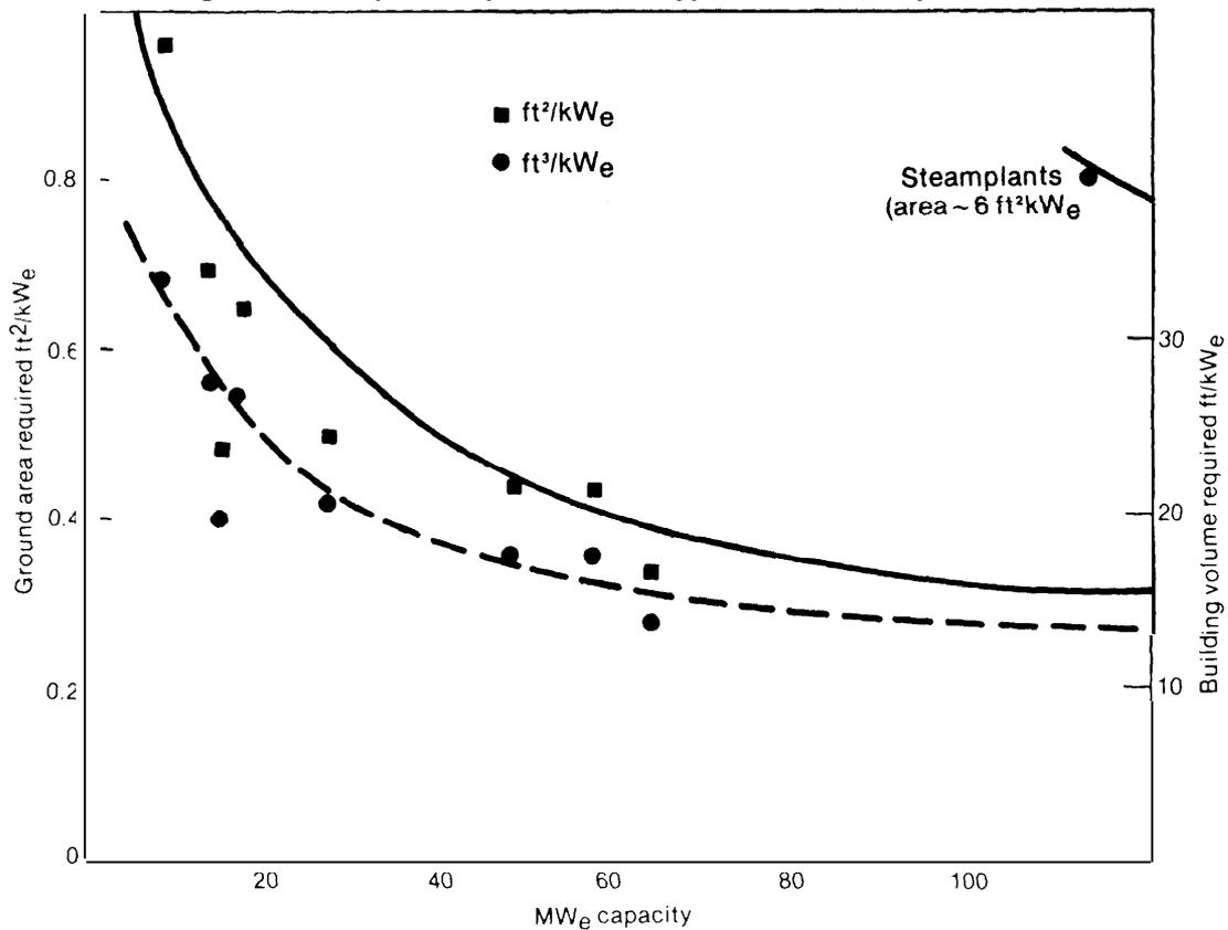
NOTE: 200 MW steamplants typically require 30-35 ft<sup>3</sup>/kW<sub>3</sub> and 6-8 ft<sup>2</sup>/kW.
