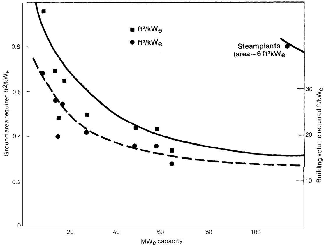
NOTE: 200 MW steamplants typically require 30-35 ft³/kW₃ and 6-8 ft²/kW.
