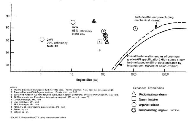
Figure IX-5.—Rankine-Cycle Expander Efficiencies
