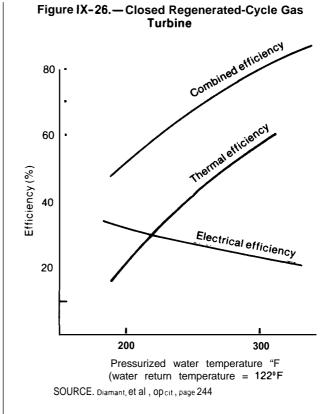
discussed above must be reduced by the efficiency of some type of power-conditioning equipment. This is because the speed of Brayton-cycle devices changes rapidly as a function of the incident power; thus, frequency control cannot be maintained in an alternator, although the Brayton-cycle device can be locked into a utility grid frequency if it is attached to utility power. In such cases, electric output power will be proportional to the energy available from the solar collector.
