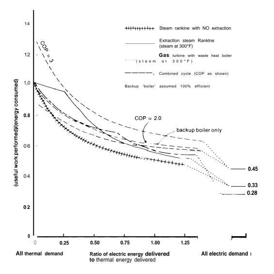
Figure IX-2.—System Performance (Ratio of Electric and Thermal Energy Produced to Energy Entering the System)
