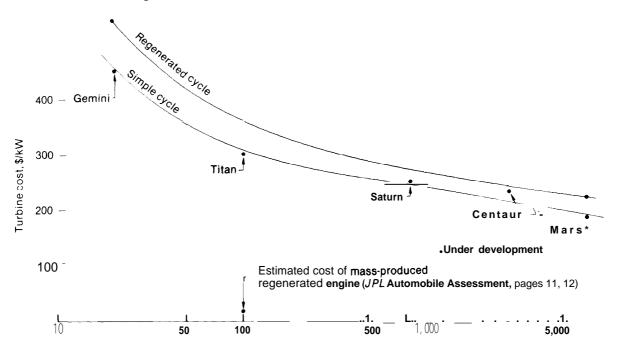
Figure IX-27.— Installed Costs of Open-Cycle Brayton Turbines
