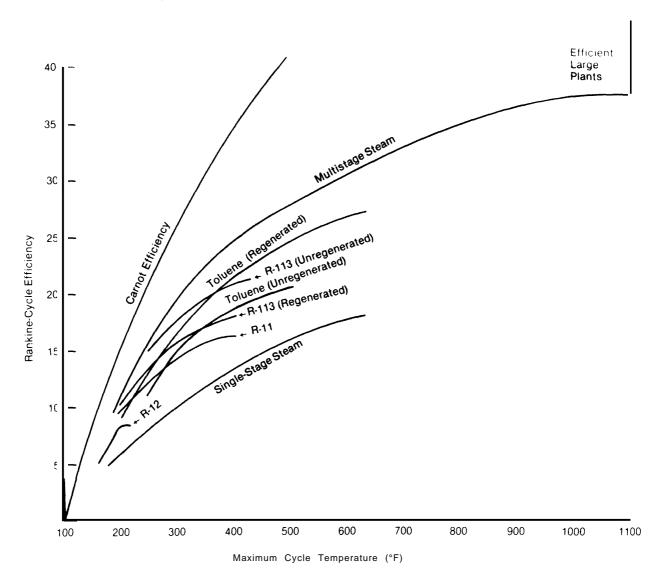
Figure IX-4.—Temperature Dependence of Rankine-Cycle Devices
