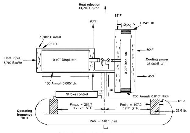
Figure IX-36.— Free-Piston Total Energy System
