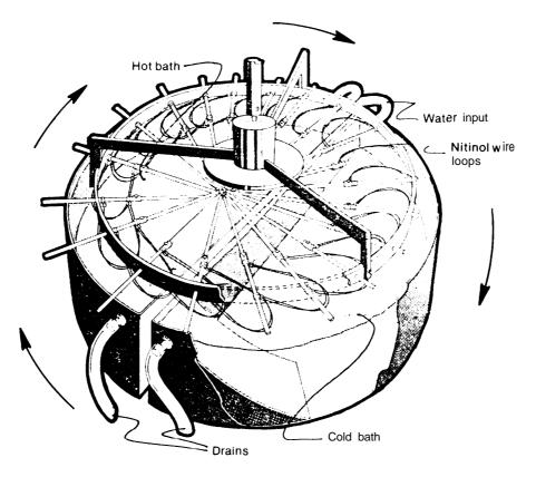
Figure IX-45.—The Nitinol Engine
