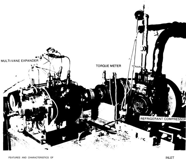
Figure IX-15.- Experimental Expander at General Electric
