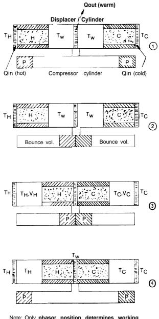
Figure IX-35. — Free-Piston Total Energy System
