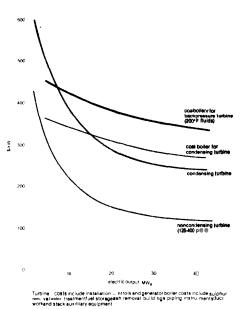
Figure IX-16.– Installed Costs of Steam Rankine Turbines erected boilers and include the cost of maintaining all of the ancillary equipment (pumps, feedwater treatment, etc.) required for the operation of the system. Approximately 10 percent of the cost shown is due to devices designed to remove sulphur and particulate from the boiler exhaust, and about 10 percent is traceable to systems for fuel-handling and storage.
