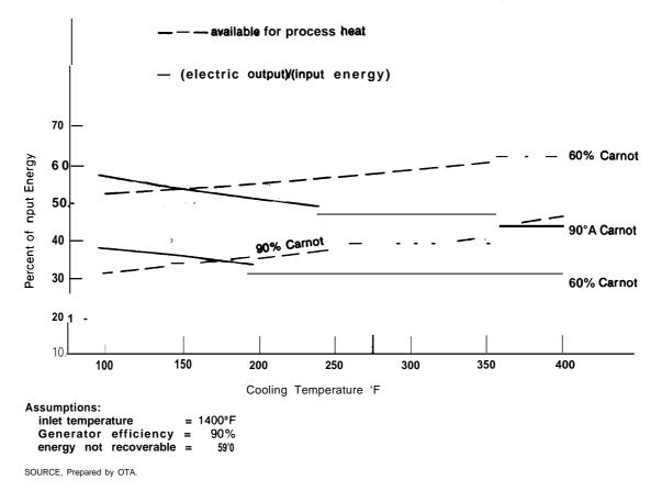
Figure IX-39.— Electric and Thermal Output of a Stirling Engine
