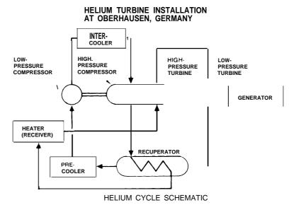
Figure IX-21 .— 50 MW Closed-Cycle Gas Turbine
