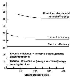
SOURCE Calculations based on performance of Rolls Royce RB.211 Gas Turbine (28,960 BHP), 2% electric efficiency loss due to backpressure
