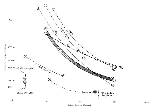
Figure IX-17.— Installed Costs of Organic Rankine Turbines
