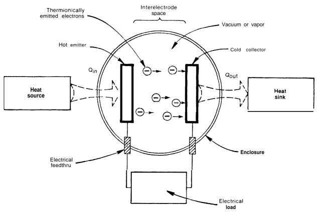
Figure IX-43.— Identification of Thermionic Converter Components
