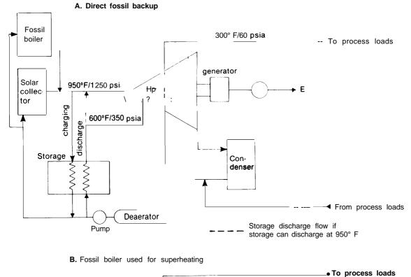
Figure IX-9.— Designs for Providing Backup Power for Solar Rankine-Cycle Systems
