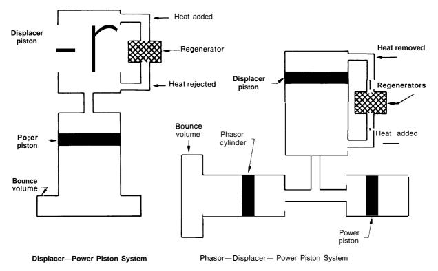
Figure IX-33.– Free-Piston Stirling and Ericsson Cycle Designs
