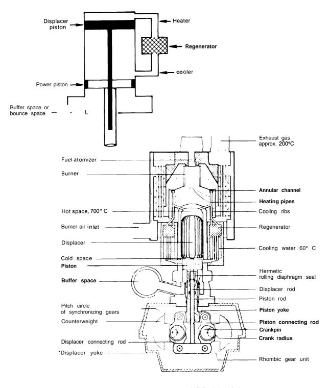
Figure IX-30.— Philips Rhombic-Drive Stirling Engine
