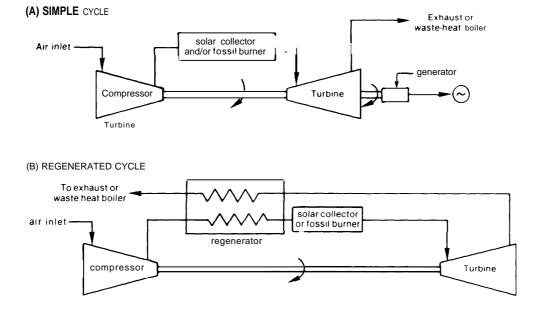
Figure IX-19.— Four Brayton-Cycle Systems Compatible With Solar Applications
