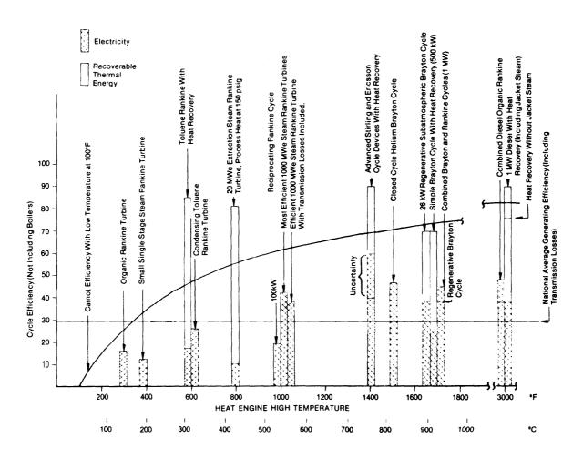
Figure IX-1 .— Cycle Efficiencies of Heat Engines
