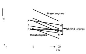
A A Stirlingengines present laboratory types B Laboratory models to be expected within a few years C Stirling engines developed for vehicles
