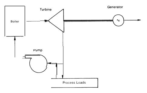
Figure IX-3.— Rankine-Cycle Devices With Heat Extraction
