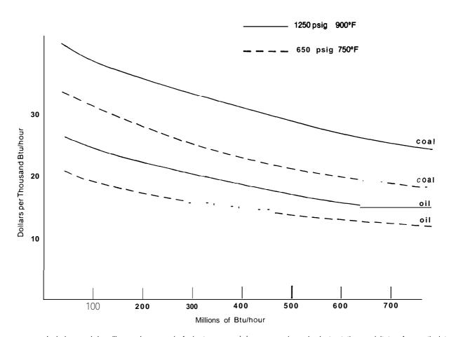
Figure IX-18.— Installed Costs of Field-Erected Boilers\*
