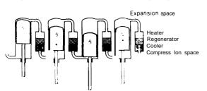
Diagram of the double-acting type Stirling engine principle of the double. acting engine There is a hot space—expansion space—at the top and a cold one—compression space—at the bottom of each of the cour cylinders shown The hot space of a cylinder is connected to the cold through a heater, a regenerator, and a cooler The pistons Pn of the cylinders move with a suitable phase shift between them In the case of four cylinders, as shown here, this shift is 90°
