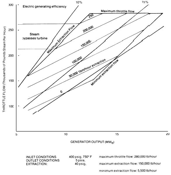
Figure IX-8.— Electric and Therma Performance of a 12.5 MW. General Electric Extraction Turbine
