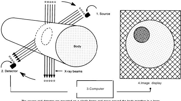
Figure 3.—Schematic Illustration of CT Scanner
