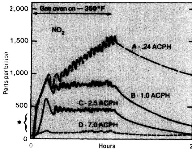
NOTE: Gas oven operated for 1-hour at 350° F.
