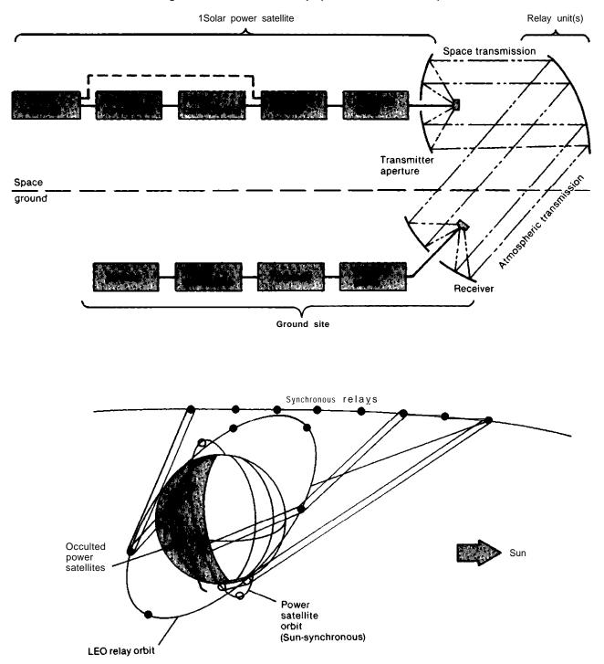
Figure 3.—The Laser Concept (One Possible Version)
