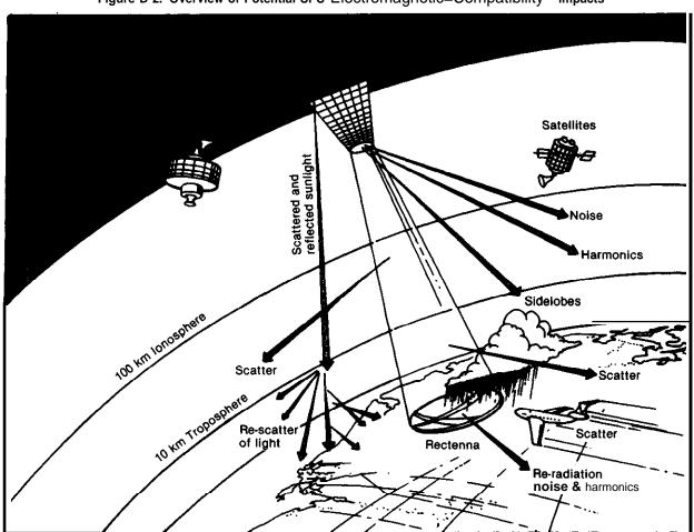
Figure D-2.-Overview of Potential SPS Electromagnetic=Compatibility impacts
