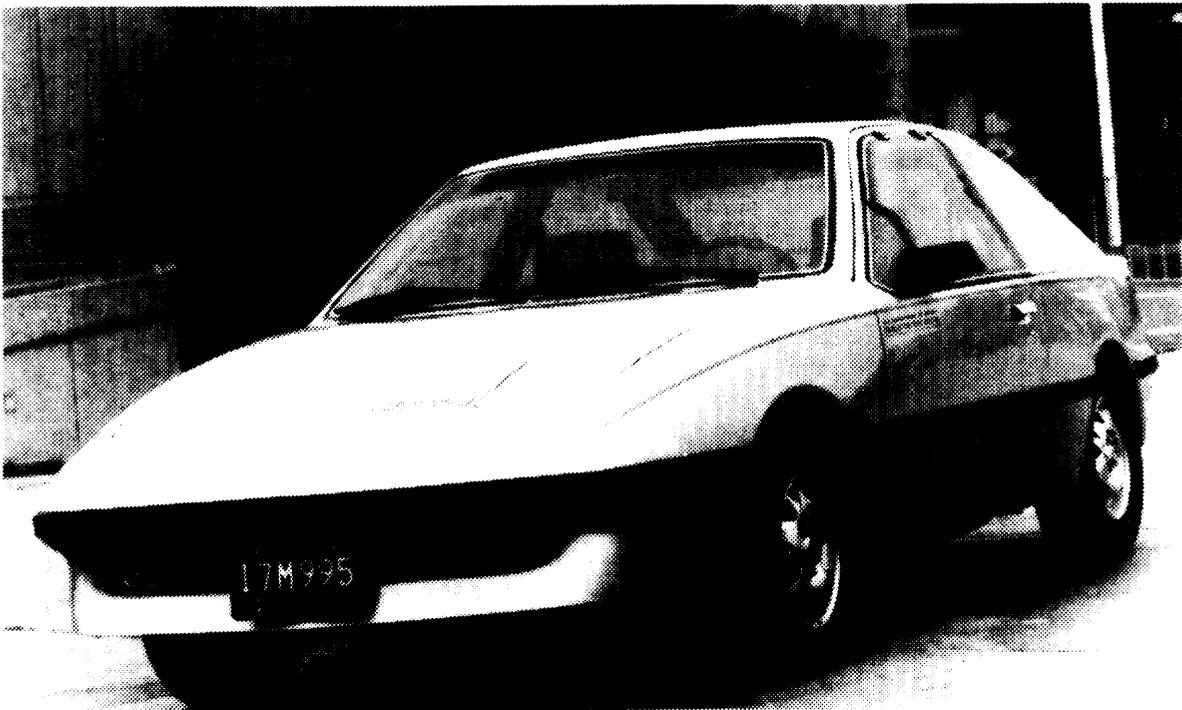
Figure 3.1 The GE/Chrysler Electric Car ETV-1
