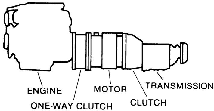
Figure 4.4 Power Train of Daihatsu 1.5-ton Hybrid Truck
