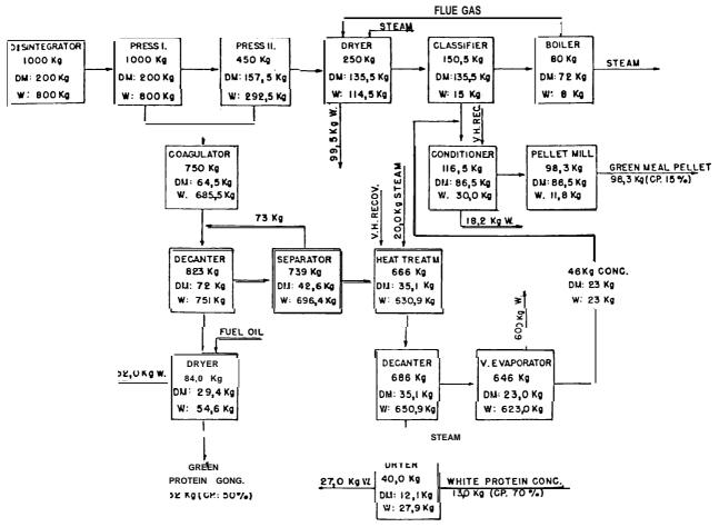
Figure 24.—Material Flow in Vepex Process
