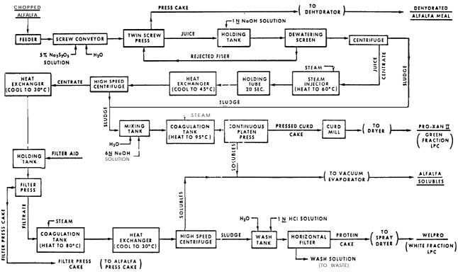
Figure 12.—The Pro-Xan Process used by the Valley Dehydrating Co.
