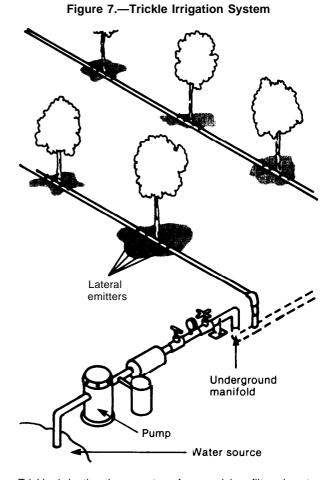
Trickle irrigation is a system for supplying filtered water directly onto or below the soil surface. Water is carried through an extensive pipe network to each plant. The outlet device that emits water onto or into the soil is called an "emitter." After leaving the emitter, water is distributed to a "wetted zone" by its normal movement through the soil. Surface application by the trickle method. Water is applied
