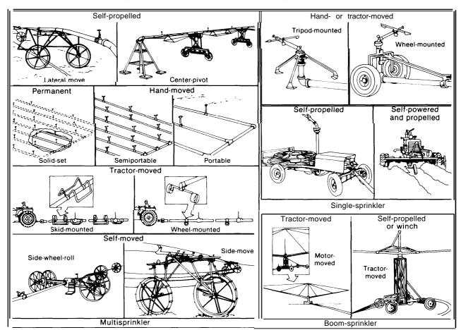
Figure 8.—Typical Types of Sprinkler Irrigation Systems
