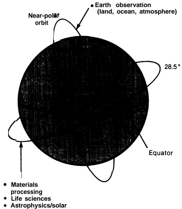
When repetitive but not full coverage of the Earth is essential, a lower inclination can be used; an orbit inclination of  $57^\circ$  is favored because it is the maximum practical inclination obtainable with a Cape Canaveral launch. It may be desirable to use infrastructure elements in several orbital planes, or perhaps to develop and employ a reusable orbital transfer vehicle (ROTV) for transportation between orbits having various inclinations, although this would be expensive.
