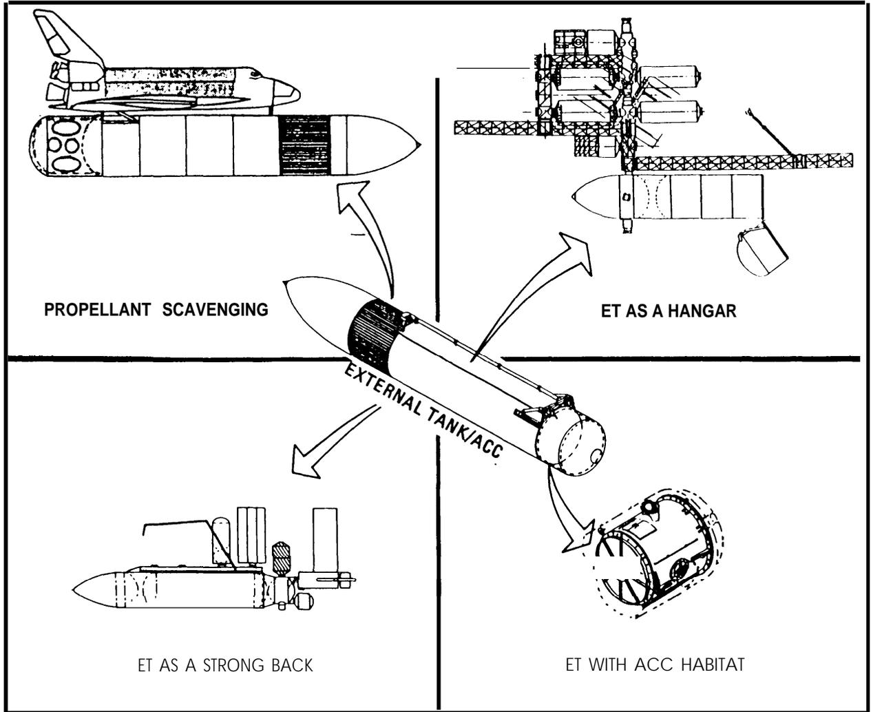
**Figure 11.—Concept of Infrastructure Utilizing Four External Tanks**
