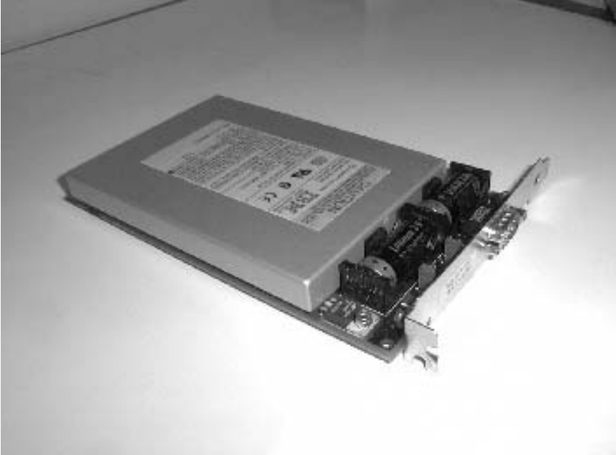
Fig. 1. – The IBM 4758 cryptoprocessor (courtesy of Steve Weingart)
