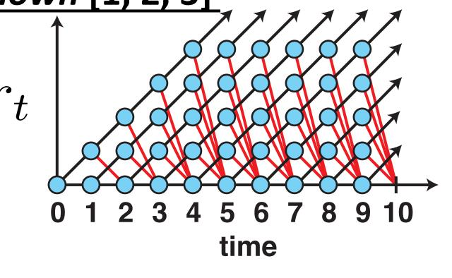
$$p(r_t|x_{1:t}) \propto \sum_{t=0}^{t} p(r_t|r_{t-1})p(x_t|r_{t-1})p(r_{t-1}|x_{1:t-1})$$
