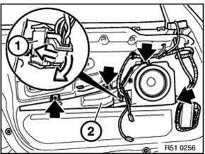
Press down connector fastener, slide lever downwards and remove connector (1) (loudspeaker).
