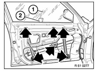
Lift door window (1) upwards and wedge into place with wooden chock (2).
