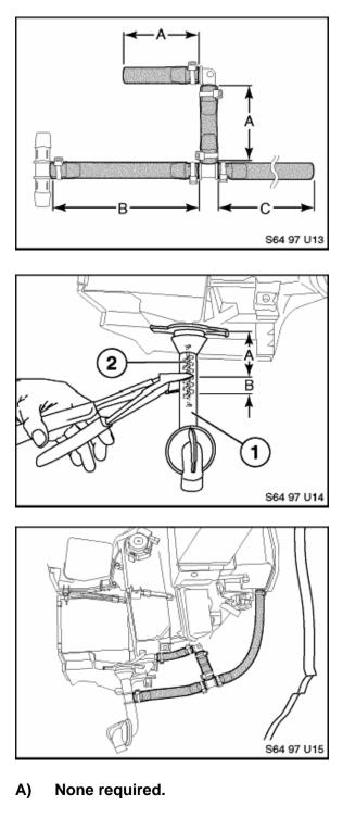
Modify the drain tubes as shown.
