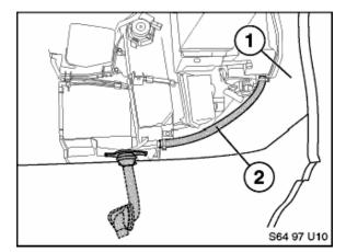
Here is the unmodified view of the fresh air drain tube(2) as seen on the passenger side. Take note of its close proximity to the firewall(1)
