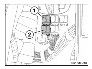
E38 Relays K36 (1) and K37 (2) in engine compartment, at bottom of E-Box
