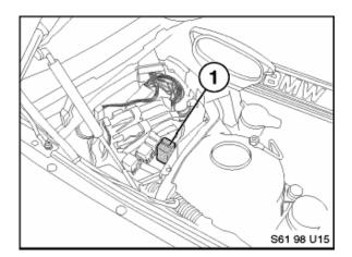
E39 from 9/97 Relay K11 (1) in engine compartment E-Box.
