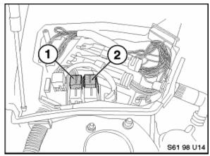
E39 to 8/97 Relays K36 (2) and K37 (1) in engine compartment E-Box
