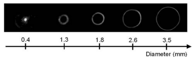
Fig. 2 Intensity image of instantaneous patterns obtained by changing the TAG lens driving frequency. Pictures were taken at a distance of 50 cm away from the lens. Frequencies from left to right are: 719 (bright spot), 980, 730, 457, 367, 337 kHz. The amplitude of the driving signal is fixed at 9.8 V peak to peak. The ring diameter is provided at the bottom of the picture. There is a half a period phase shift between the spot and the ring pattern
