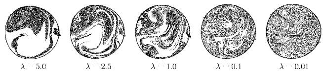
FIG. 10. The mixing patterns at the exit of the channel as a function of the viscosity ratio. ( Ca=0.025, Re=6.6, \Lambda=0.76 , Grid: 1024 \times 64 .)
