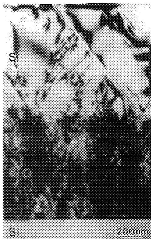
FIG. 5. Defect distribution in sample 1039 with a similar growth condition as in sample 1052. Note that the density of stacking faults in the Si capping layer decreases drastically.
