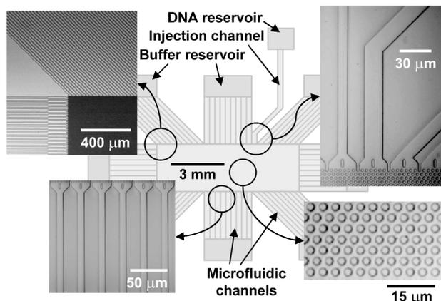
**Figure 1.** Structure of the microfabricated device illustrating the sieving matrix integrated with the microfluidic channels. The post array is 3 mm × 9 mm, and the posts are 2 μm in diameter, 2 μm apart, and 2 μm tall. A single channel connecting to the DNA reservoir injects DNA through a 28-μm opening. The many microfluidic channels connecting to buffer reservoirs produce uniform electric fields over the sieving matrix by acting as electric-current injectors<sup>17</sup>.
