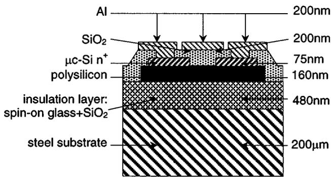
FIG. 1. Schematic cross section of a polysilicon top-gate transistors on a passivated steel substrate, showing materials used and their thickness.
