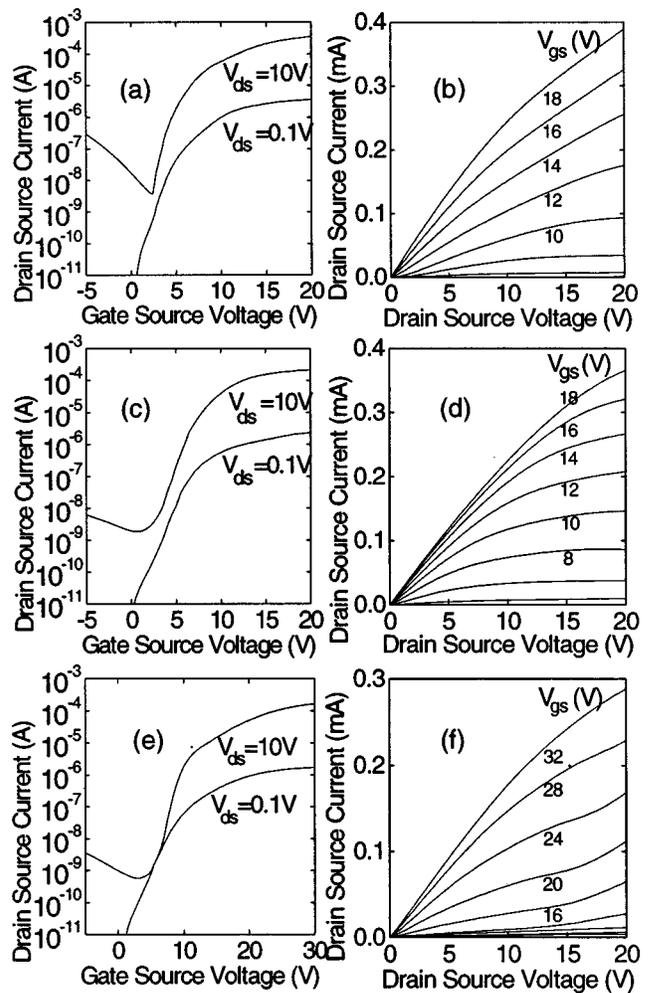
FIG. 2. (a) Transfer characteristics and (b) output characteristics of a top-gate TFT made by crystallization at 650 °C of silicon on steel,  $V_{ds}$  and  $V_{gs}$  are the drain source and gate source voltages. (c), (d) and (e), (f) are transfer and output characteristics of top-gate TFTs made by crystallization at 600 and 700 °C of silicon on steel. All TFTs have a dimension of  $W/L = 180 \mu\text{m}/45 \mu\text{m}$ .
