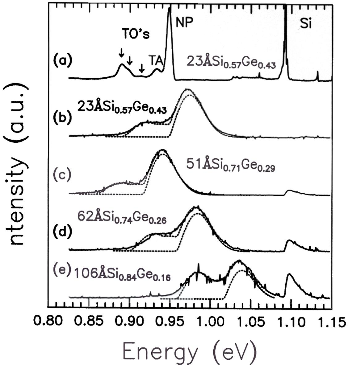
Figure 4.4: PL spectra of strained  $\langle 110 \rangle$  Si/Si<sub>1-x</sub>Ge<sub>x</sub>/Si quantum wells measured at (a) 4K and (b)-(e) 77K. The dotted lines in (b)-(e) are the theoretical fitting of electron hole plasma model and the no-phonon component of the model. The onsets of the no-phonon lines at the low energy side are the bandgaps of the quantum wells,  $E_{g,PL}$ .
