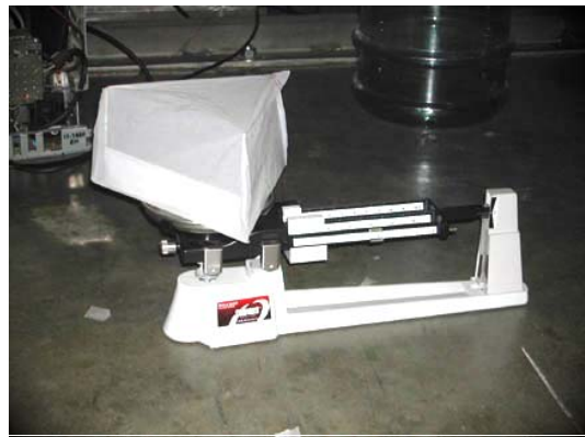
Figure 4 — The enclosed lifter in this picture did not move the balance when it was activated.
