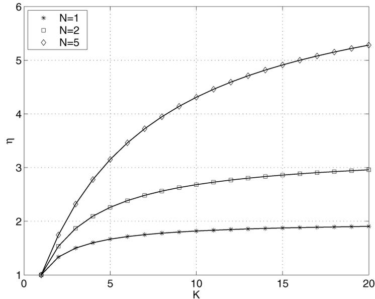
Fig. 5. Bandwidth expansion factor of TDMA over superposition coding versus the number of users  $K$  for the Rayleigh-fading case.
