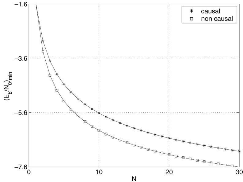
Fig. 2.  $(E_b/N_0)_{\min}$  in decibels versus  $N$  for the Rayleigh-fading case.
