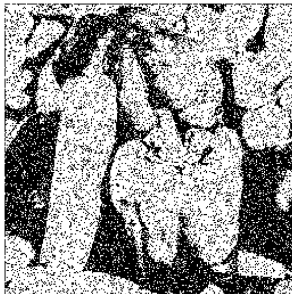
Fig. 3. Noise corrupted image, generated by passing the original signal through a BSC(0.15).
