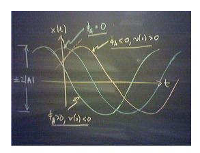
Figure 2.4: Position as a function of time for the harmonic oscillator, from Eq (2.113). Note that when the initial velocity is zero the phase  $\phi_A$  also is zero. Positive initial velocities correspond (in this notation) to negative phases, and vice versa.
