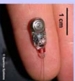
Figure 1. Example of a transmitter that is currently used in bird research that could be tracked from a low-orbit satellite
