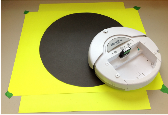
Figure 3: The Create microworld consists of a mobile robot constrained by its behaviour to explore a small space. Four downward facing sensors on the front of the robot detect the color difference on the paper sheets. This boundary serves as a virtual wall, and the sensors serve as whiskers. At each timestep, an observation vector indicates contact (1) or non-contact (0) with the “wall” and the action selects a direction of rotation for each wheel.
