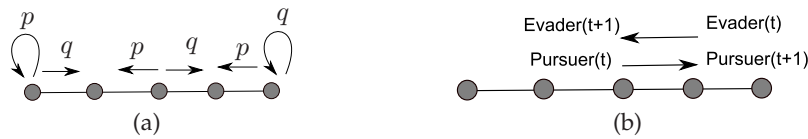
Figure 1: (a) Target's motion model. Here p = (1 - q) . (b) The pursuer will miss the target if they cross each other.
