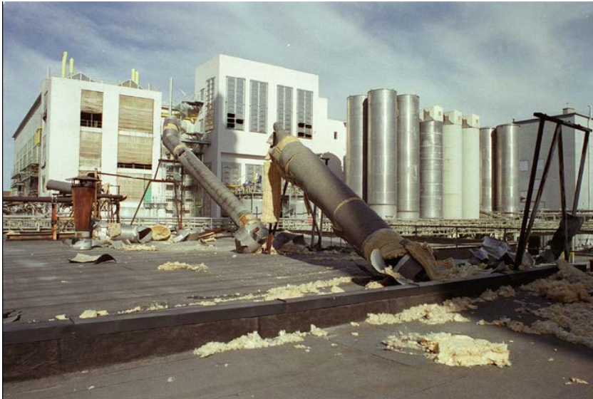
Hydrogen Explosion in a Pipe. Norsk Hydro Ammonia Plant, Norway, 1997
