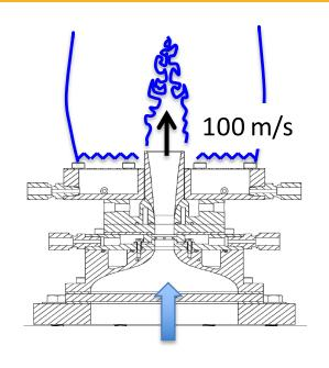
Mean velocity up to 100 m/s  $u'/S_L$  up to 246  $L_x/\delta_L$  up to 215  $Re_T$  = up to 100,000
