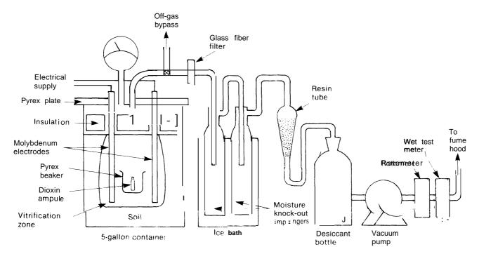
Figure 2-10—Bench-Scale ISV Unit Tested With Dioxin-Contaminated Soil From the Jacksonville, AR Superfund Site in February 1987
