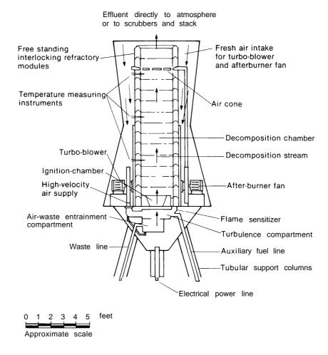
Figure 2-3-Vertically Oriented Liquid Injection Incinerator
