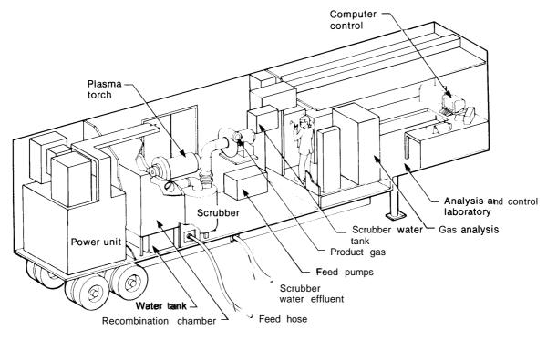
Figure 2-8—Westinghouse Environmental Services' Pyroplasma Waste Destruction Unit
