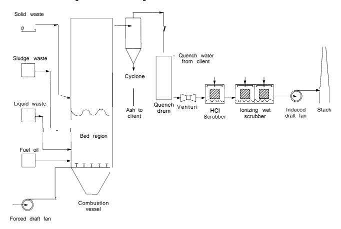
Figure 2-4-Schematic Diagram of the Waste-Tech Incineration Process
