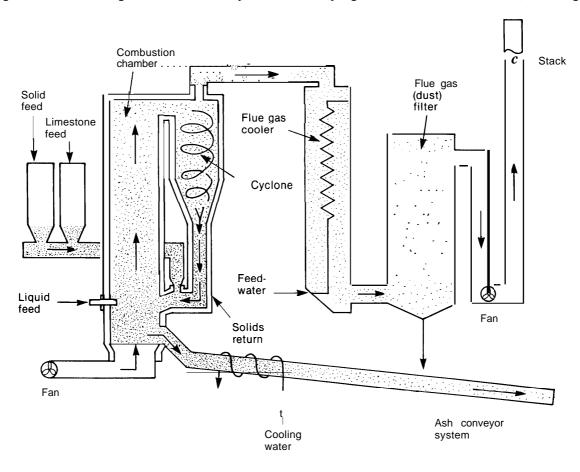
Figure 2-5—Circulating-Bed Combustion System Offered by Ogden Environmental Services, San Diego, CA
