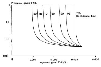
Figure D-I-Confidence Limits on the Probability of Death or Life-Threatening Injury, Given the BFS Test is Passed
