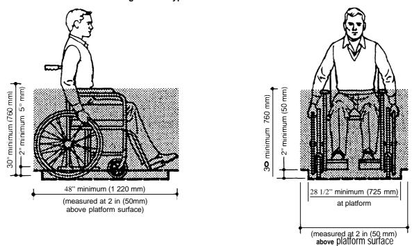
Figure 4-I—Typical Wheelchair Dimensions
