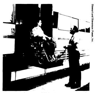
A passenger leaves an OTRB using an exterior-style lift.
