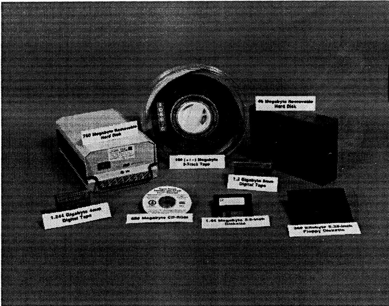
A common form of hardware incompatibility is that of the media used to store data. The picture shows a frustrated user's exhibit of the many media on which he received remotely sensed Earth data during Operation Desert Storm.
