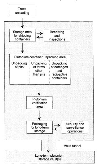
Figure 4-2-Conceptual Design of a DOE Plutonium Storage Facility
