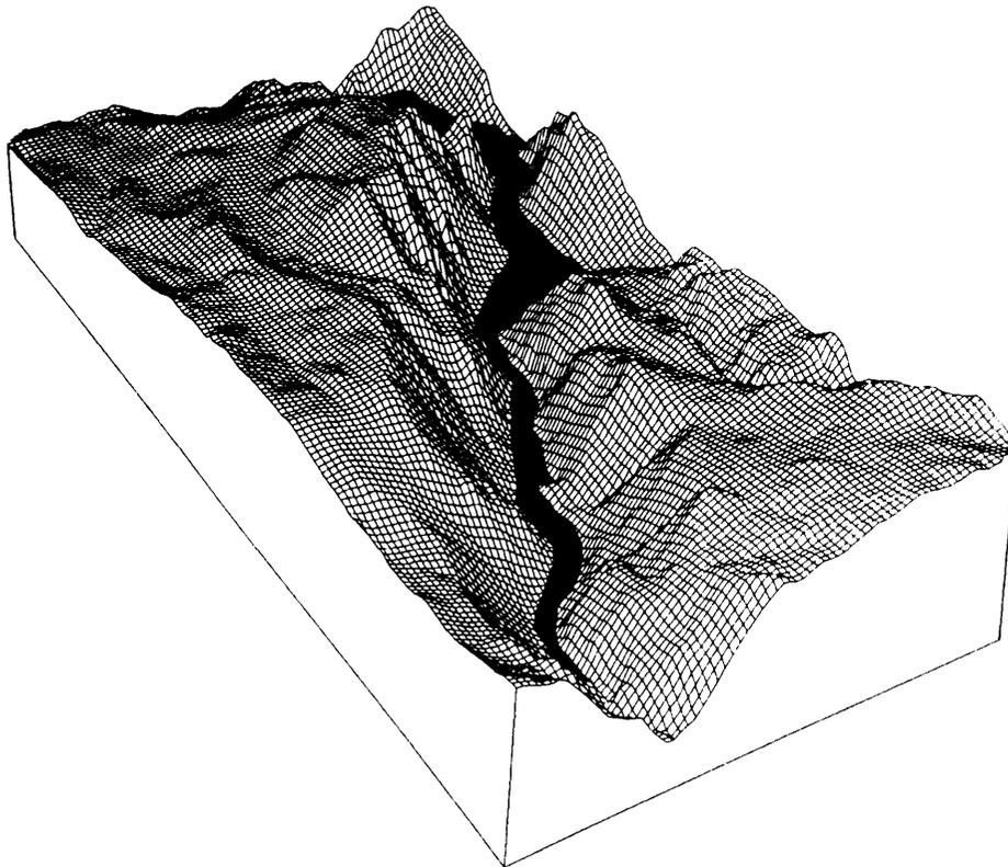
The U S Geological Survey prepared this digital elevation model of the Hetch Hetchy Canyon in Yosemite National Park, California using aerial photographs
