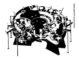
The Large Helical Device (a stellarator) under construction in Japan is estimated to cost about \$1 billion.
