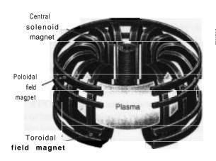
Tokamak magnets. A tokamak uses three types of magnets. Toroidal field magnets create a 'container" for the plasma, while poloidal field magnets keep the plasma centered and stable. The central solenoid magnets induce an electric current in the plasma.
