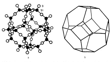
Figure 1.—Simple Polyhedron of Silicate and Aluminate Tetrahedra
