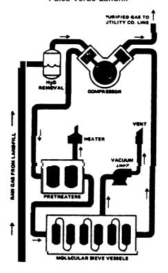
percent carbon dioxide is fed to two pretreatment vessels to remove moisture, hydrogen sulfide, and mercaptans. The dry gas is then routed through three parallel columns packed with pellets of dehydrated chabazite/erionite and carbon dioxide is removed by adsorption on the zeolite. Approximately 1 million cubic
