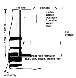
Mined geologic disposal will use a system comprised of engineered barriers (the waste package and the mined repository) and naturally occurring barriers (the host rock formation and the chemical and physical properties of the repository site itself) to provide long-term isolation of waste from the biosphere. Three decades of extensive study have revealed no insurmountable technical obstacles to the development of mined geologic repositories, provide suitable sites are found.
