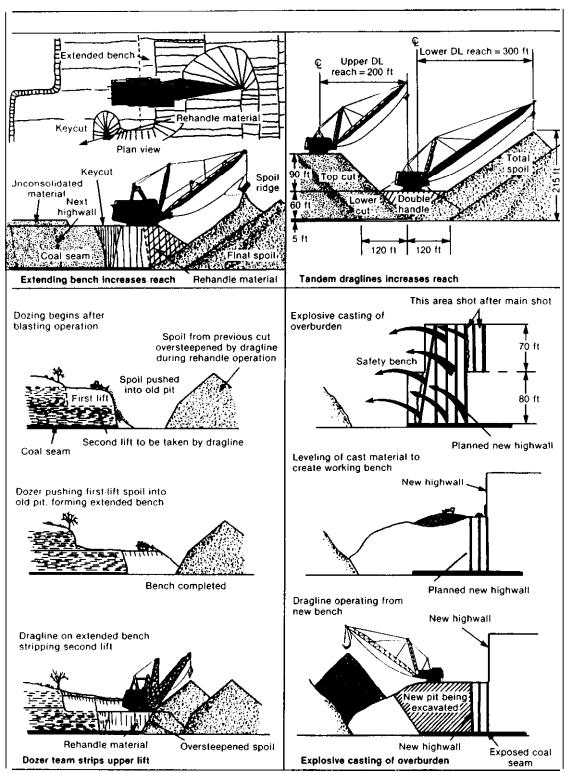
Figure 3-8.— How To Help Draglines Reach Deeper Seams
