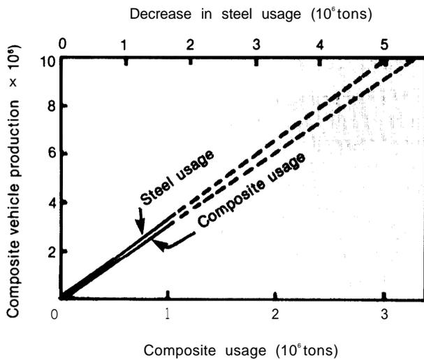
Increase in composites usage and associated decrease in steel usage for various production volumes of composite-intensive vehicles. Assumes 1,000 lb. of steel is replaced by 650 lb. of composites in a typical vehicle weighing 2,700 lb. that contains 1,600 lb. of steel.
