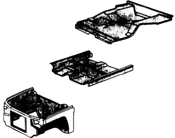
**Figure 7-20(b).—Typical Assembly of Underbody, Bodyside Assemblies, Etc. into the Completed Steel Body Shell**
