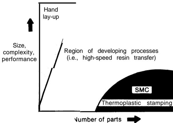
Viable commercial processes must be able to produce a large number of high performance parts.
