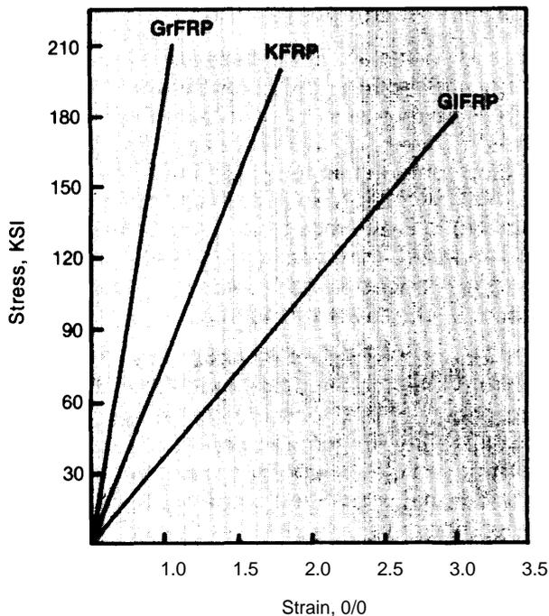
The linearity of the curves means that these composites behave as brittle materials during fracture (cf fig. 7-6). There is no plastic region to absorb crash energy.
