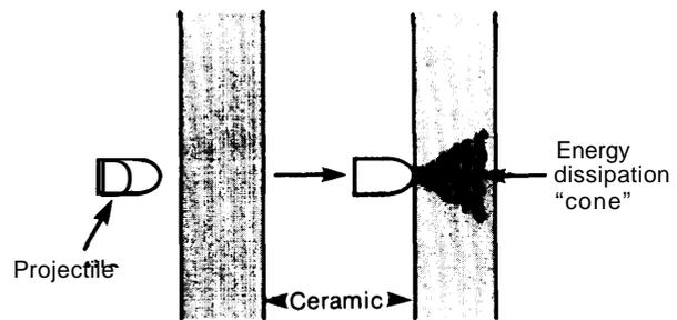
Energy absorption occurs in ceramics and brittle PMCs by spreading local impact energy into a high-volume cone of fractured material.
