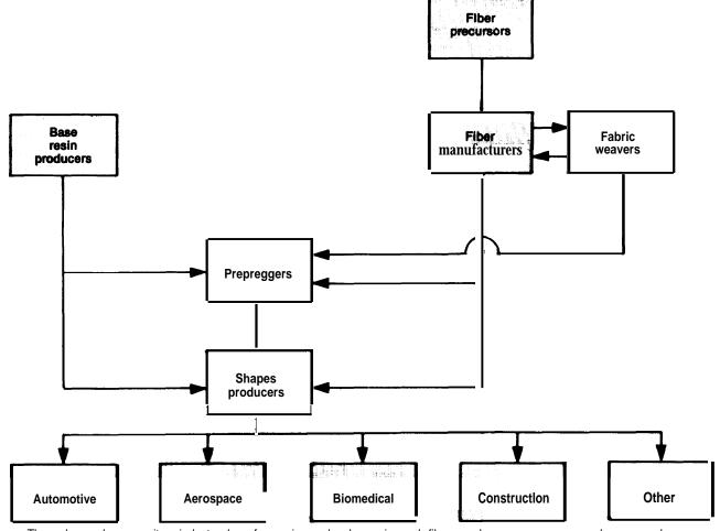
Figure 9-2.-Structure of the Advanced Composites Industry
