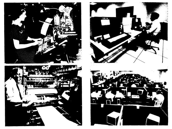
Clockwise from top left: a hot type scene at GPO, circa 1940s; GPO operator using electronic photocomposition equipment; GPO operators using keyboard input terminals; and the Congressional/ Record coming off the press (photo credit: U.S. Government Printing Office).
