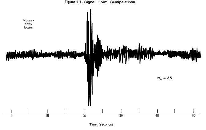
Seismic signal from a 0.25 kt explosion at the Soviet test site near Semipalatinsk. Recorded 3,800 km away at the NORESS seismic array in Norway on July 11, 1985. The signal to noise ratio is about 30 indicating that much smaller explosions could be detected even at this great distance.
