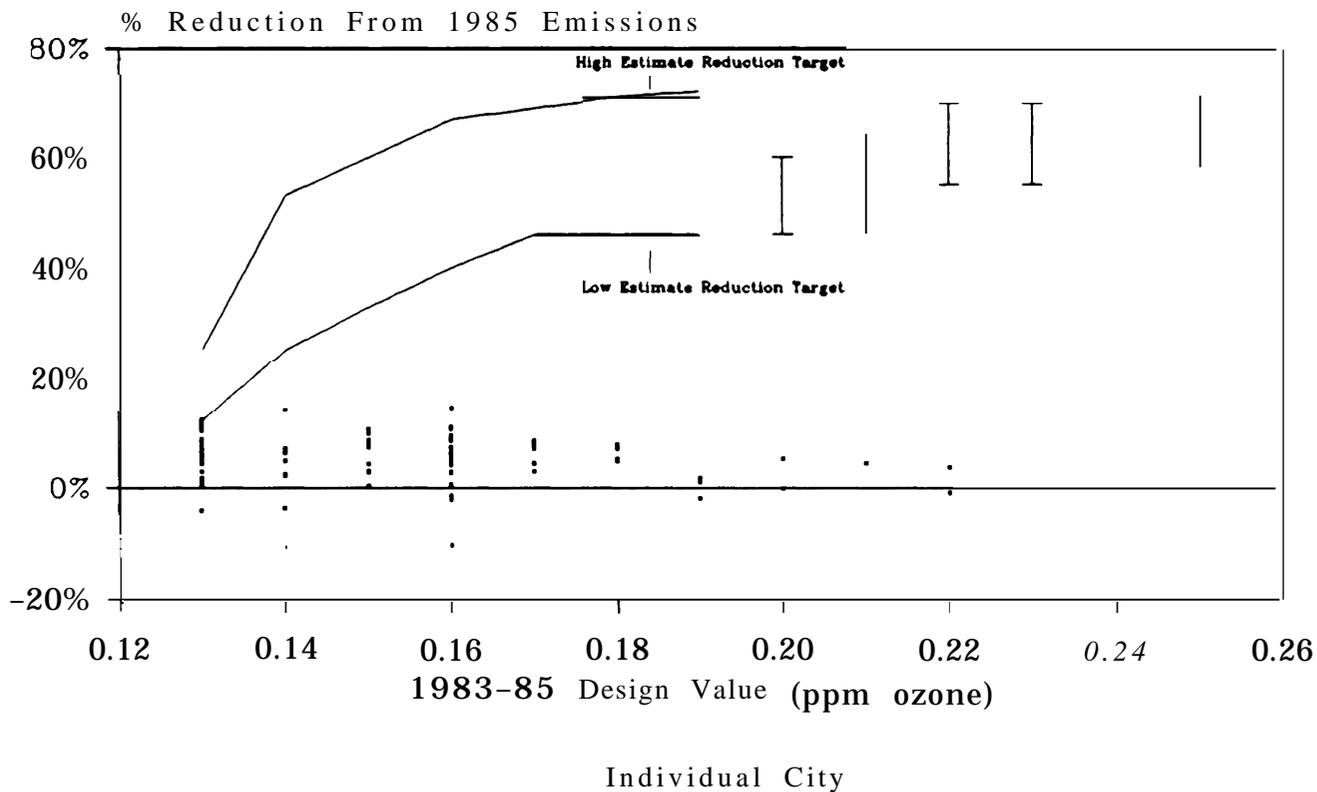
Figure 3-11. Volatile Organic Compound (VOC) Emissions Reductions Between 1985 and 1993, Assuming No Change from 1985 VOC Regulations.
