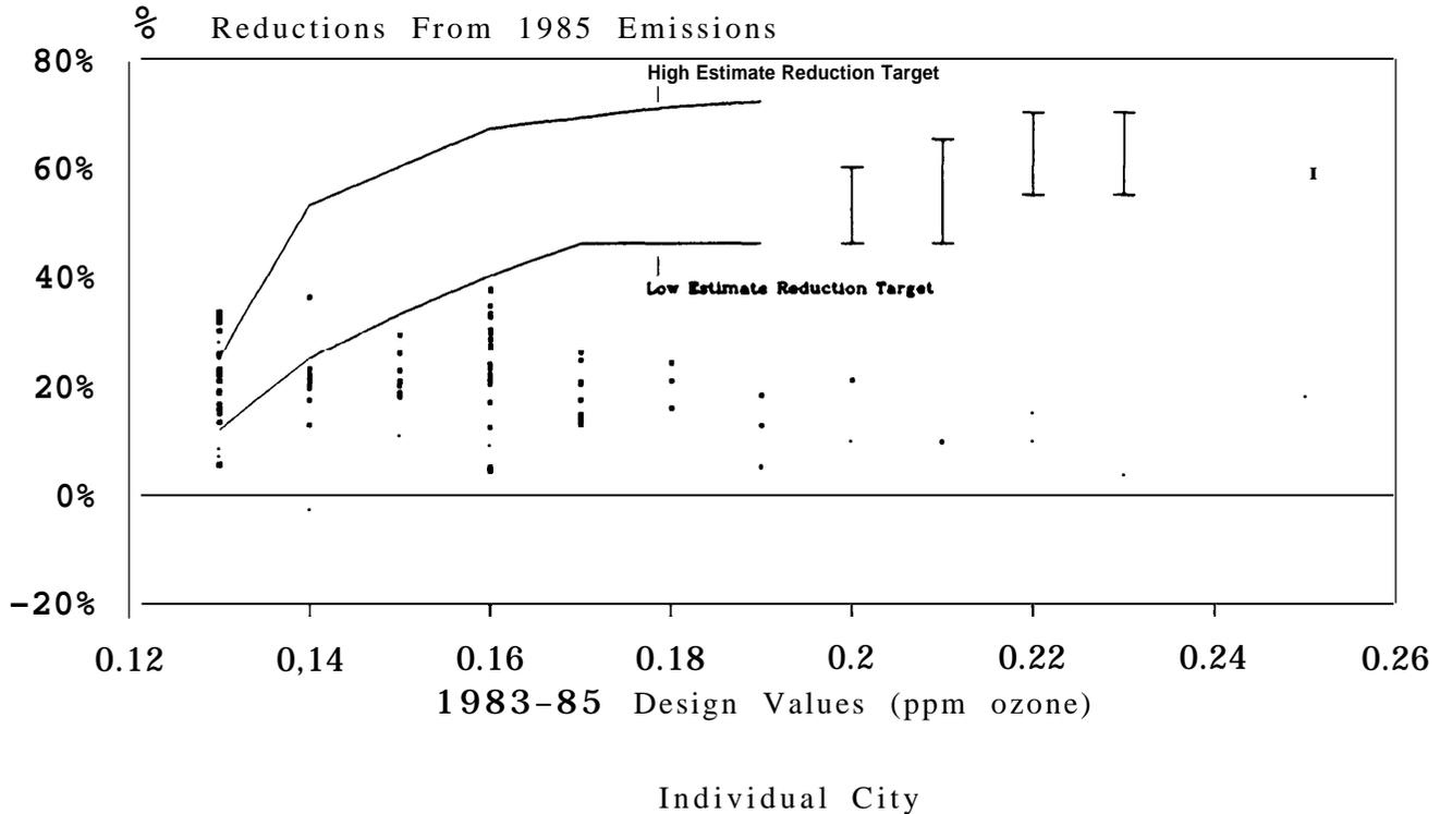
Figure 3-15. Volatile Organic Compound (VOC) Emissions Reductions Between 1985 and 2003, Including All Mobile and Stationary Source Control Strategies.
