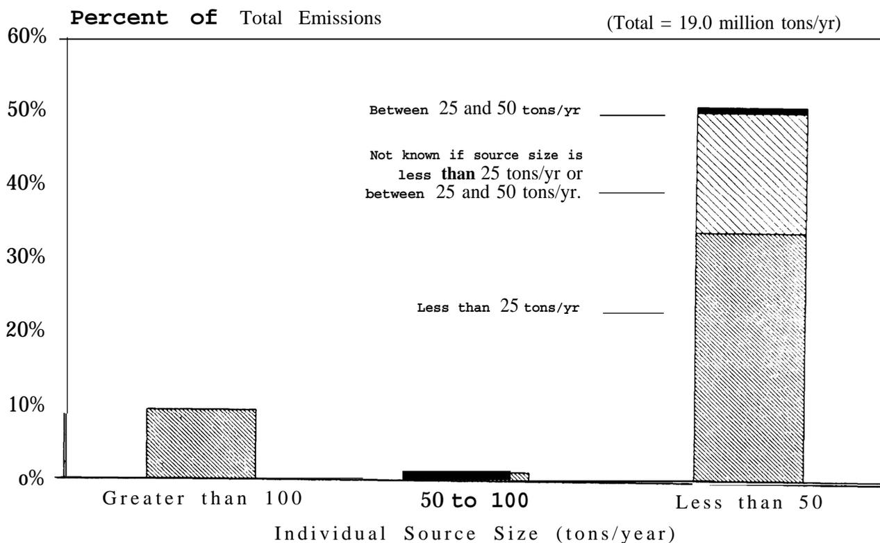
Figure 3-6. Stationary Source Emissions of Volatile Organic Compounds (VOCs) as a Percentage of the Total Emissions Inventory, By Size of the Individual Source.
