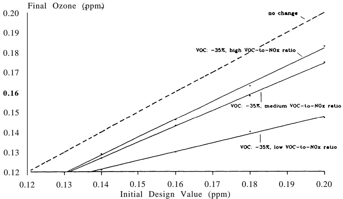
Figure 3-2. Ozone concentrations predicted to result when VOC emissions are reduced by 35 percent, with no change in NO<sub>x</sub> emissions levels. The three solid lines indicate the ozone concentrations predicted to result in cities with low, medium and high VOC to NO<sub>x</sub> ratios. The dashed line illustrates the “no control” case, i.e. the final ozone concentrations are the same as the initial design values.
