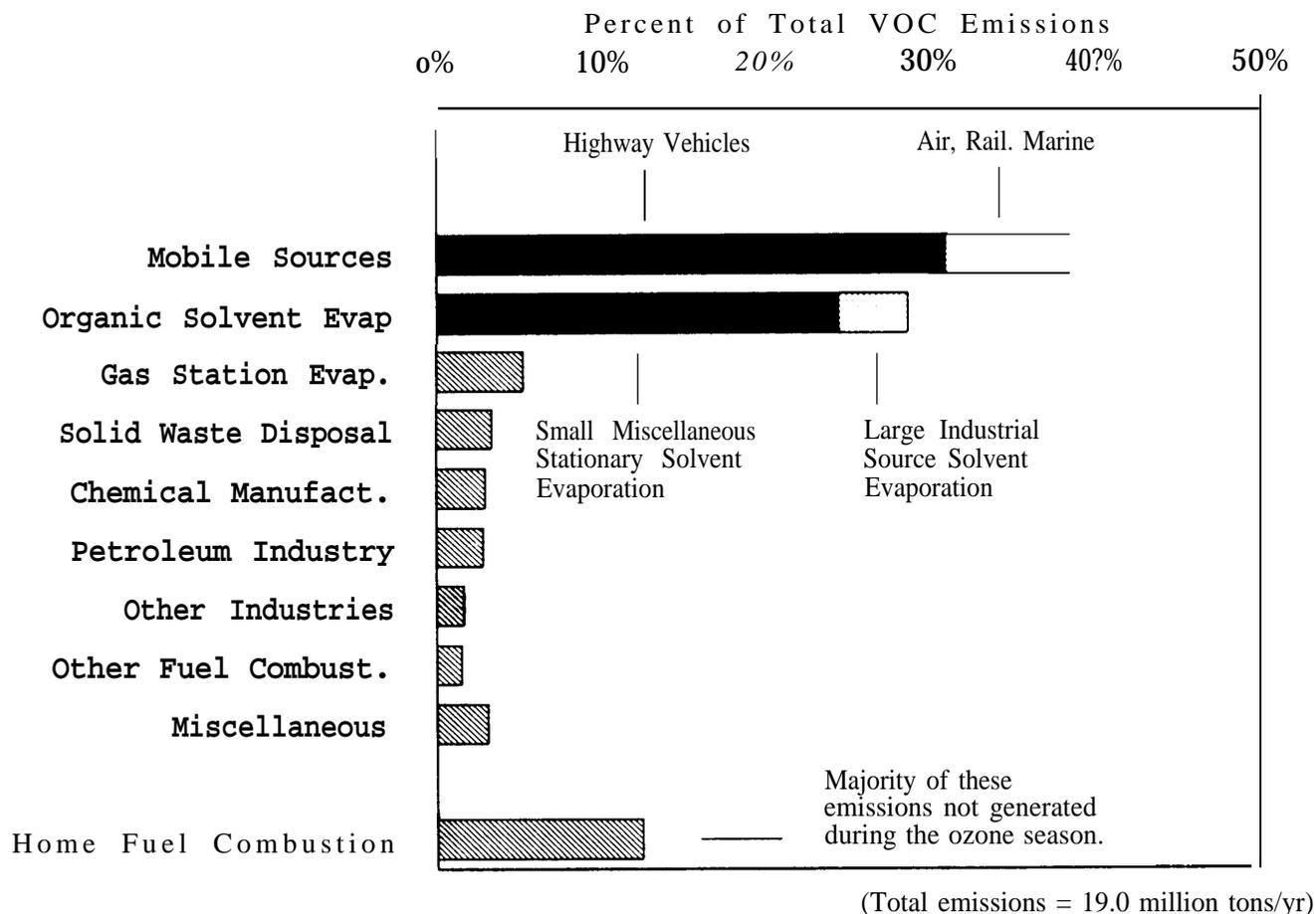
Figure 3-4. Volatile Organic Compound (VOC) Emissions by Source Category in 1985. Source: OTA, from EPA's National Emissions Data System (NEDS)
