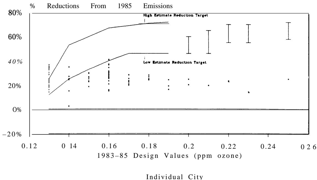
Figure 3-14. Volatile Organic Compound (VOC) Emissions Reductions Between 1985 and 1993, Including All Mobile and Stationary Source Control Strategies.
