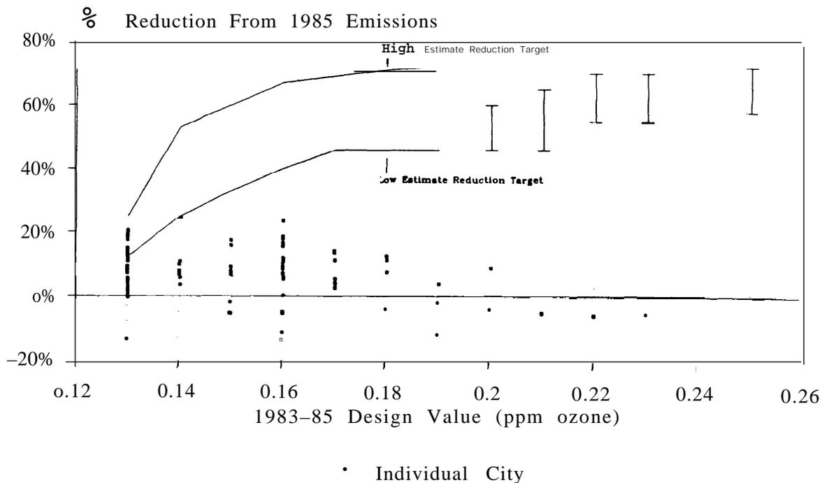
Figure 3-13. Volatile Organic Compound (VOC) Emissions Reductions Between 1985 and 2003, Including Onboard and Additional Fuel Volatility Controls.
