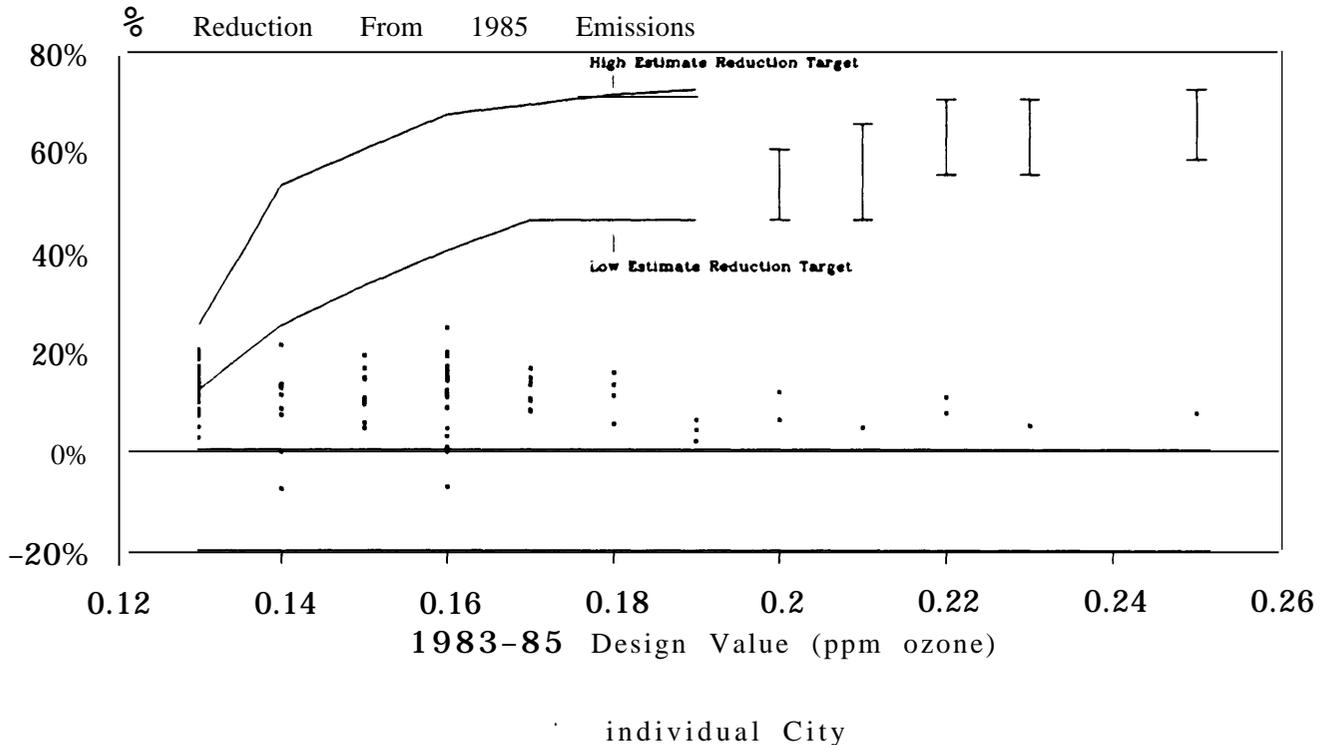
Figure 3-12. Volatile Organic Compound (VOC) Emissions Reductions Between 1985 and 1993, Including Onboard and Additional Fuel Volatility Controls.
