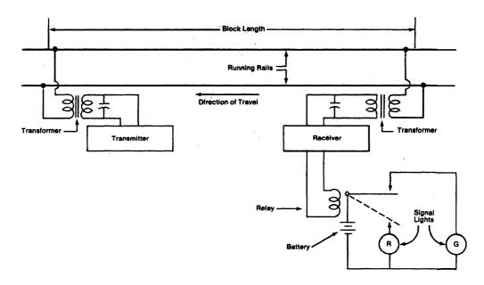
FIGURE B-3.—Simple High-Frequency A.C. Track Circuit
