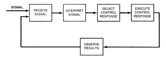
**FIGURE 2.—Generalized Control Process**
