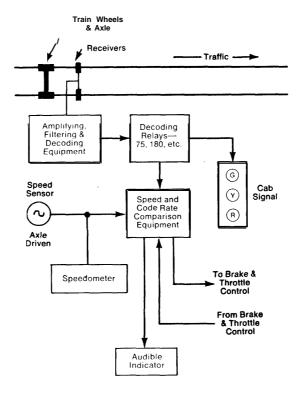
FIGURE 7.-Cab Signal System With Automatic Overspeed Protection
