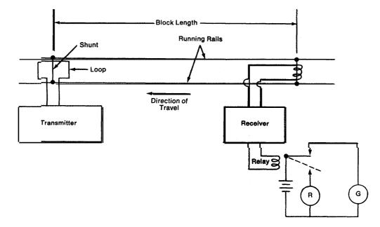
FIGURE B-4.—Alternate High-Frequency A.C. Track Circuit
