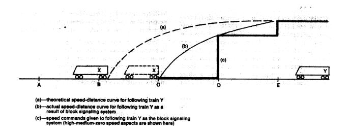
FIGURE A-2,-Train Separation in a Conventional Block Signaling System
