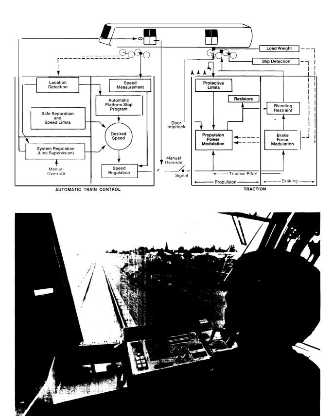
FIGURE 8.—Automatic Train Operation System
