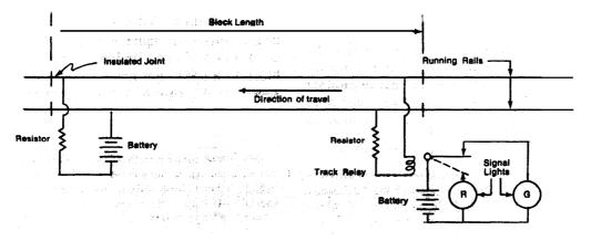
FIGURE B-1.-Simple D.C. Track Circuit
