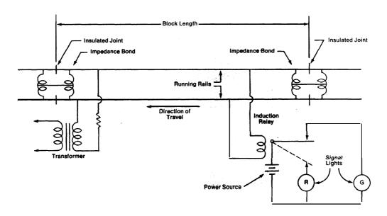
FIGURE B-2.—Simple Power-Frequency A.C. Track Circuit
