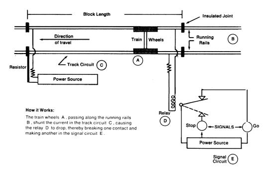
FIGURE 3.—Simple D.C. Track Circuit
