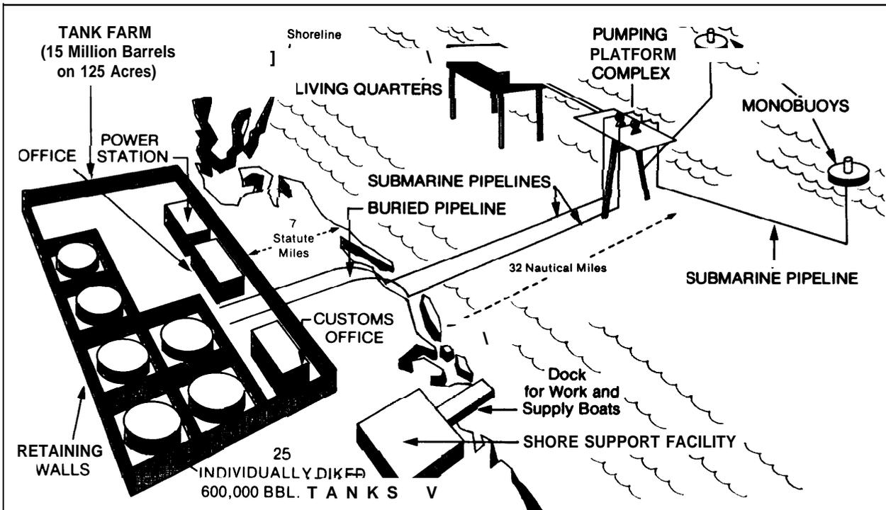
tank holds 600,000 barrels of crude; therefore, the initial two-buoy port discussed here would require 25 tanks on 125 acres of land to store a 10-day supply of 1.6 million barrels per day. If the port were expanded to 3.5 million barrels per day capacity, 58 storage tanks on 250 to 300 acres of land would be required.
