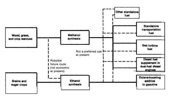
Figure 3.—Sources and Uses of Alcohol Fuels From Biomass
