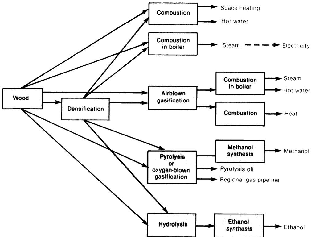
For each of these uses, the wood can be used directly or it can be pelletized first. Pelletization reduces the moisture content and improves the solid fuel handling characteristics. This enables pellets to be transported longer distances and easily ground to a small particle size for relatively automatic operation of facilities. These can be important features for some users.
