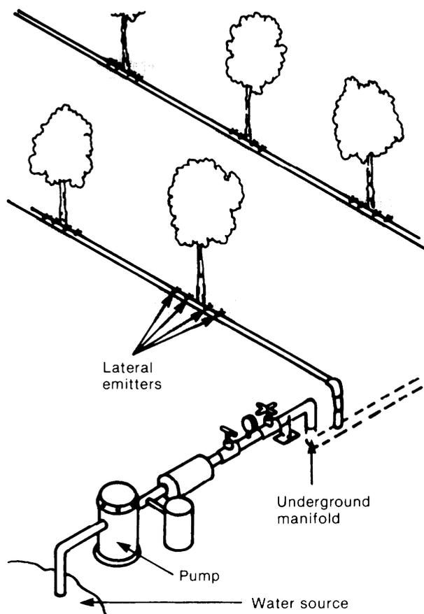
Drip irrigation systems usually consist of a network of small-diameter plastic tubing along each row or between pairs of crop rows. Water is discharged through uniformly spaced small openings in the tubing or through emitters, nozzle-like devices that regulate water flow from lateral lines into the soil. Filtration equipment, provisions for fertilizer and pesticide injection, a fertilizer holding tank, and hardware to regulate water pressure are usually included as part of the system.
